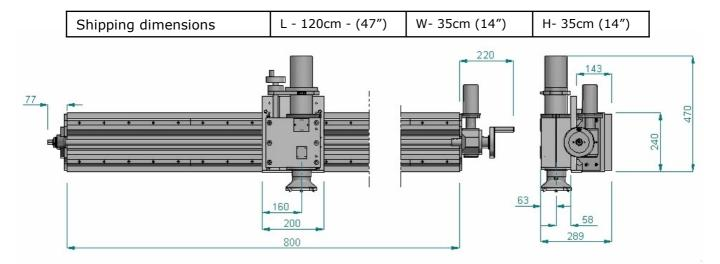
The machine is supplied complete with toolkit including air filter lubricator and hose connection (when required), all required bolts and storage / shipping box, CE certificate, Packing list and Manual
