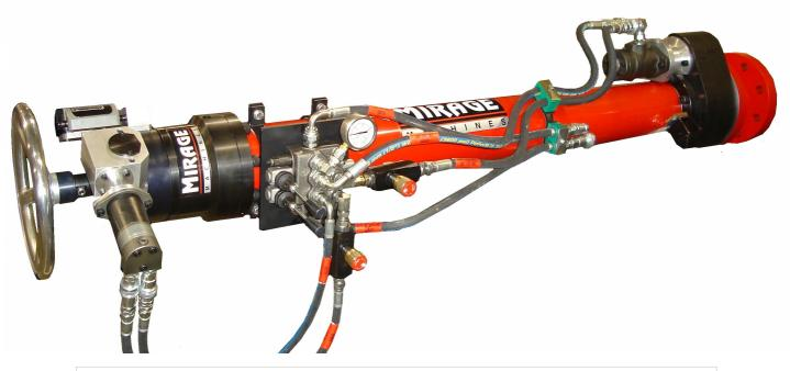
A Hot Tapping machine with a working pressure capacity of 5000 p.s.i maximum and can Hot tap from Ø3 – 16" specifically designed for all pipeline intervention and wellhead maintenance.
